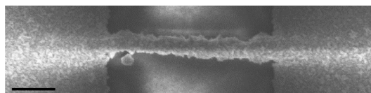
Figure 5. SEM image illustrates gold enhancement, which results in formation of a homogeneous gold wire along the rolling circle product. The gold wire is about 300 nm wide. Scale bar is 1 \mu\text{m} .
